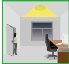
With movement and insufficient natural light. The light switches on (100% brightness).
