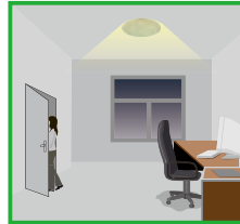
When no movement is detected the sensor enters "Hold-Time" period. After "Hold-Time" has elapsed the sensor enters "Stand-By-Time" period. Dimmed light output (10%/20%/30%/50%).
